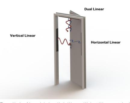
The combination of three polarizations - Vertical Linear and Horizontal Linear mounted on the sides, Dual Linear on top of the doorframe - guarantees a 360° reading coverage regardless of the tag orientation.
