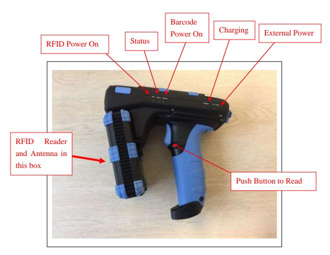
Figure 4-2 CS108-2 Reader Left Side View
