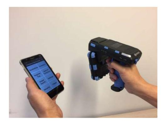
Note: Smart phone and CS108 can only be paired via the App provided. They DO NOT pair via the normal Bluetooth Device connection page of the OS. Therefore, install the App first and pair the CS108 from inside the App.
